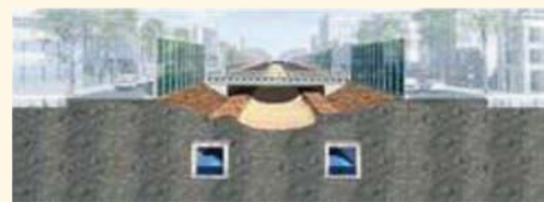
Stage 4: Sewer and bridge construction (September 2004)
